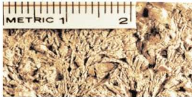
Fig. 2. Close up view of ice impressions in paste of frozen fresh concrete. The ice crystal formations occur as unhardened concrete freezes. They do not occur in adequately hardened concrete. The disruption of the paste matrix by freezing can cause reduced strength gain and increased porosity.
