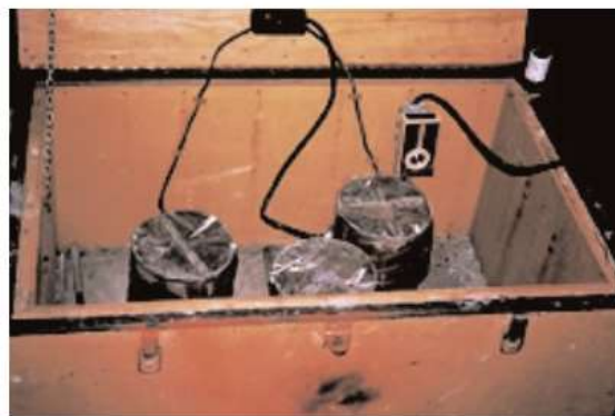
Fig.13. Insulated curing box with thermostat for curing test cylinders. Heat is supplied by electric rubber heating mats on the bottom. A wide variety of designs are possible for curing boxes.
